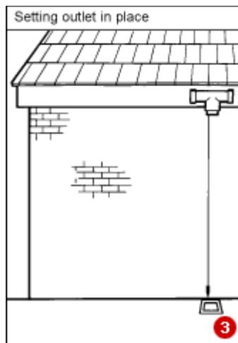
Using 25mm x 5mm (1in x No. 10) screws, fix the outlet to the fascia, allowing for the fact that the far end of the gutter must be higher than the outlet by 10mm for every 6m of gutter (a fall of 1:600).
