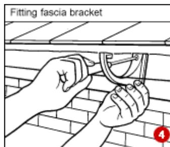
Tie a string line tightly from the end fascia bracket(s) to the outlet and use this as a guide for installing the remaining fascia brackets, which should be placed no more than 1m apart, working outwards from the outlet. Screw each bracket to the fascia with two or three gutter screws (4).
