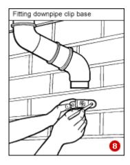
Continue to fit the remainder of the pipe in the same way, fitting the open end of one pipe into the socket of the pipe below, allowing a 10mm gap between the end of the pipe and the bottom of the socket for expansion in warm weather.
